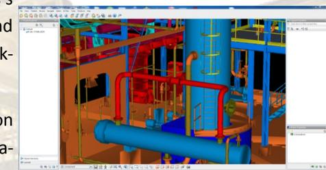
Solinas seamlessly handles revision, bends, jacketed spools, and transfers of components between isometrics.
